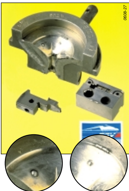
Repair and resurfacing of tools and moulds.
